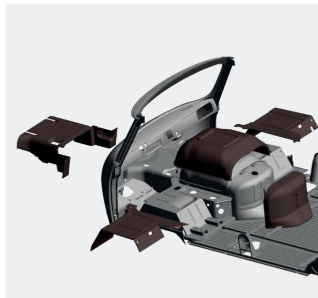
Due to improved engine noise insulation and body noise and vibration insulation, a more comfortable environment within the vehicle has been achieved. Noise insulation with pile surface covering improves acoustic comfort and interior cabin decor.
