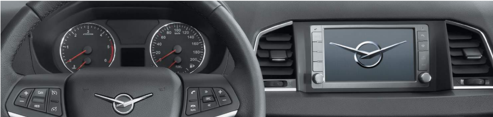
Multimedia 7-inch touch-screen display with adjustable tilt angle is located at the same level as the revamped white instrument cluster, providing comfort and safety when driving
