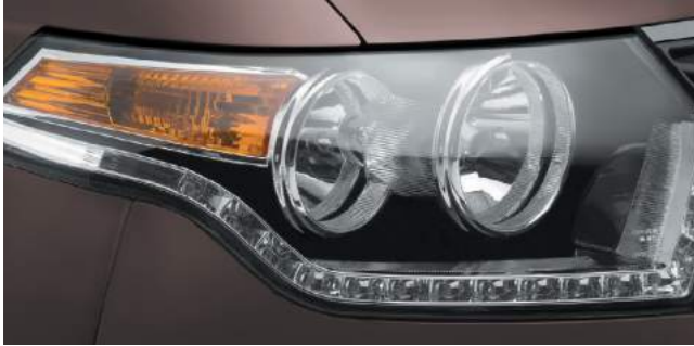
Headlamps with LED daytime running lights
