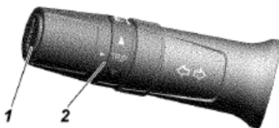
Fig. 3.6. Scheme of moving the left lever of the understeering switch when controlling the direction indicators and headlights (see item description in the text)
