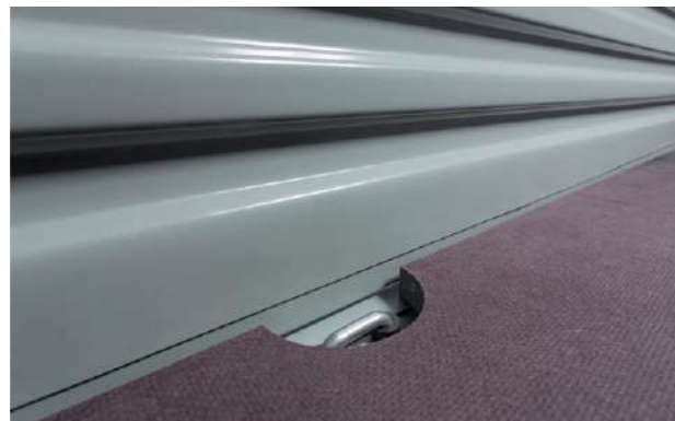
Durable plywood flooring, with flush lashing points to secure freight
