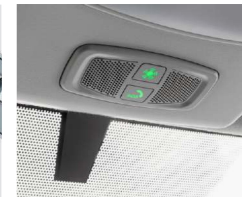
Terminal of ERA-GLONASS emergency system
