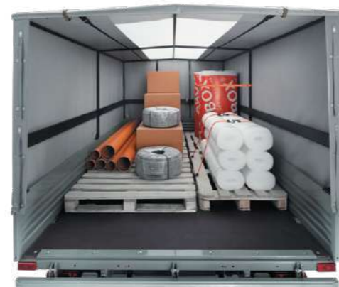
Translucent panels in the curtain box roof allow for daylight, no extra light needed
