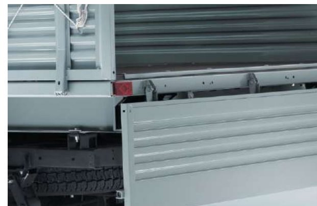
Rear lights indicating the vehicle dimensions with its tailgate open
