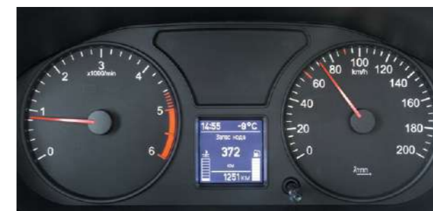
On-board computer operated via the left steering column switch
