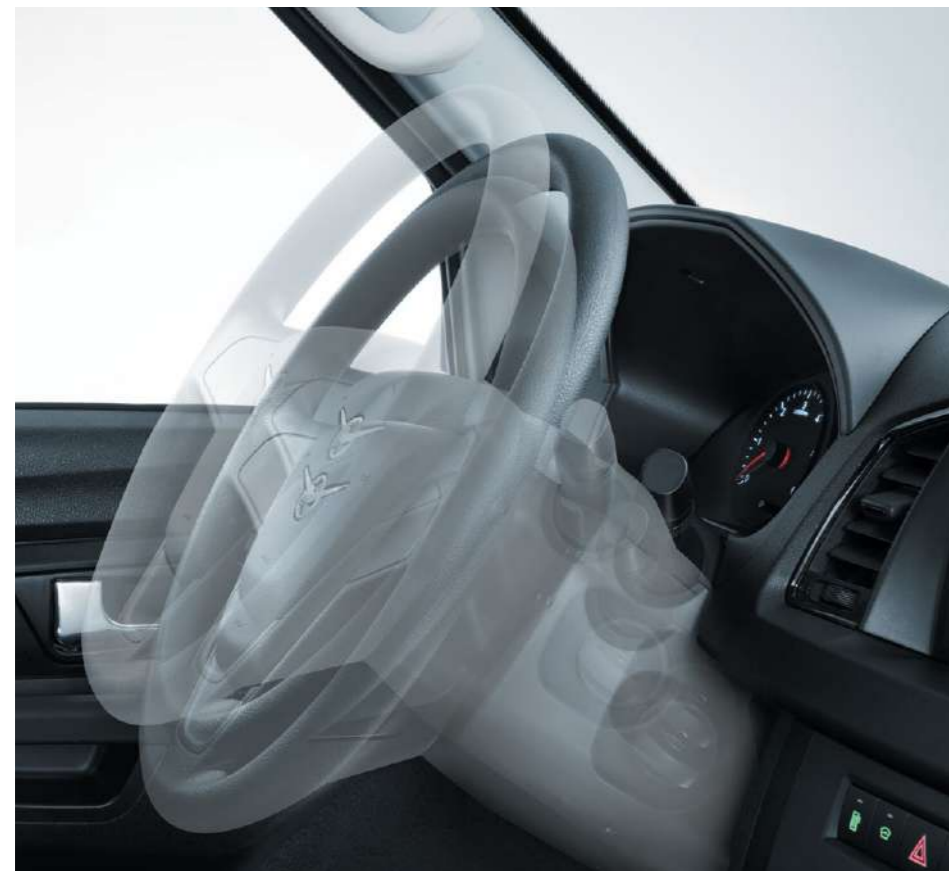
The steering wheel can be adjusted for height and for depth
