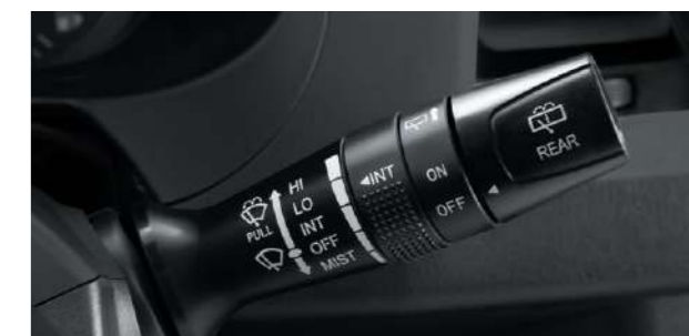
Right steering column switch with adjustable windscreen wiper delay
