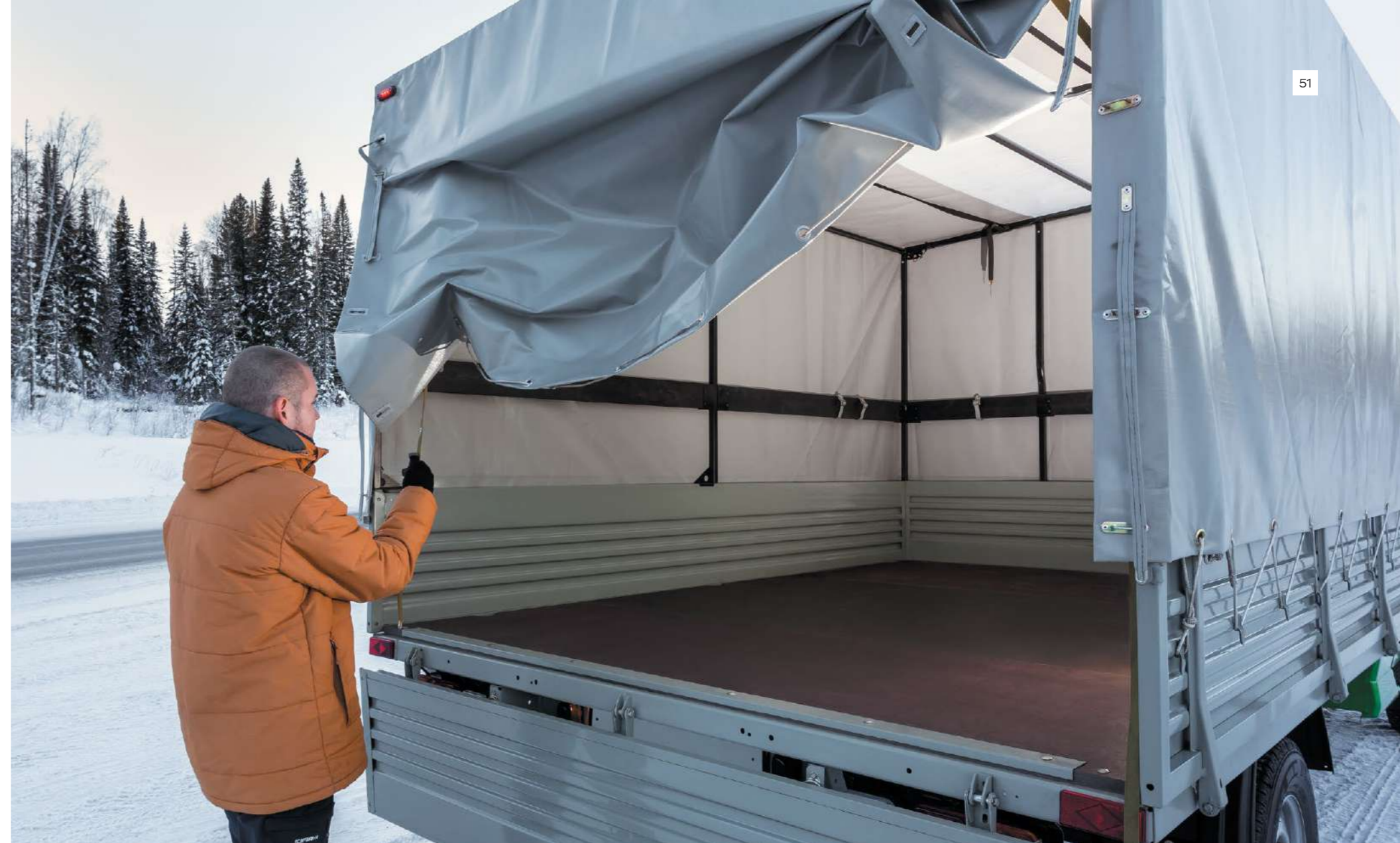
By pulling the straps, you can easily raise the curtain flap by yourself, with no tools used, and fix it open up with hooks
