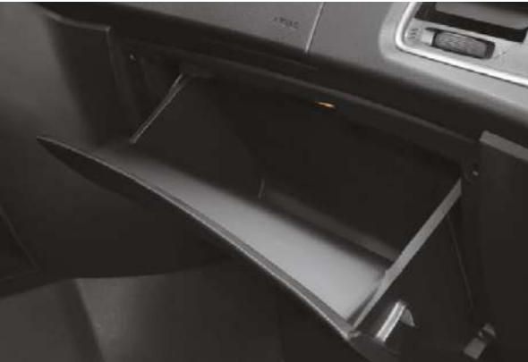
Cooled glove box with USB port
