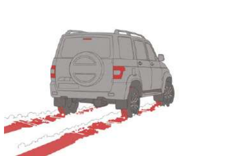
Off-Road mode is switched on with a special button on the central console to improve braking efficiency on loose surfaces
