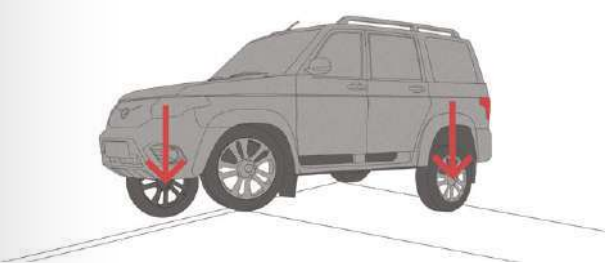
Traction Control System (TCS) serves as electronic inter-wheel differential lock and optimizes traction on drive wheels
